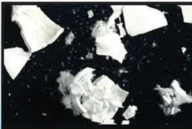
Magnification of PavIX/Sofix crystals that block moisture transmission
