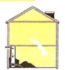
The moist air is then vented to the outside of your home through a duct while being replaced with a flow of drier, fresh air drawn downward from the upper levels of your home.
