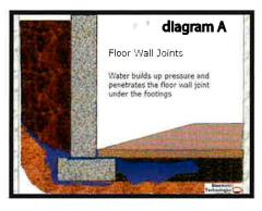
where the foundation footing meets the foundation wall. Water seeks the point of least resistance and therefore, will come in on the joint over the footing and under the foundation wall and then straight to where the floor meets the wall. This is particularly true if there are no floor cracks or penetrations in the cement floor in the basement. (see diagram A)
